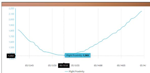
It is expected that the proximity graph will usually be a curvature which indicates the flights are nearing till a point and then moving apart.
