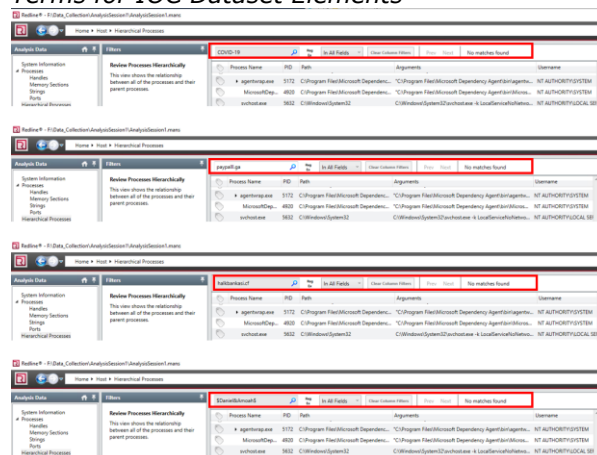
Figure 9 Forensics Analysis of VM Server2 Memory with Unencrypted Dataset Match Details
